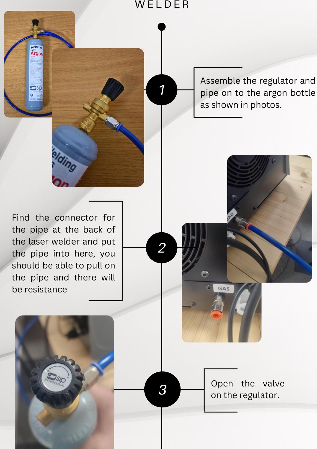
Add to the gas setting on the laser welder and move the pipe inside the laser to the working area.
