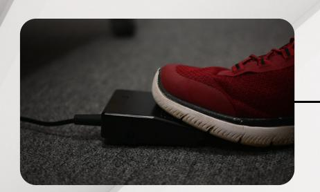
When you press the pedal to fire the laser you should hear gas enter the chamber then press the pedal again and the laser will fire. Each time you go to press the pedal it will release more gas first.
